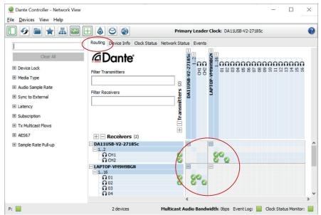
It is also possible to change the settings of the DA11USB-V2 under the "Device Info" screen in the Dante Controller software. To do so, select the "Device Config" menu.
