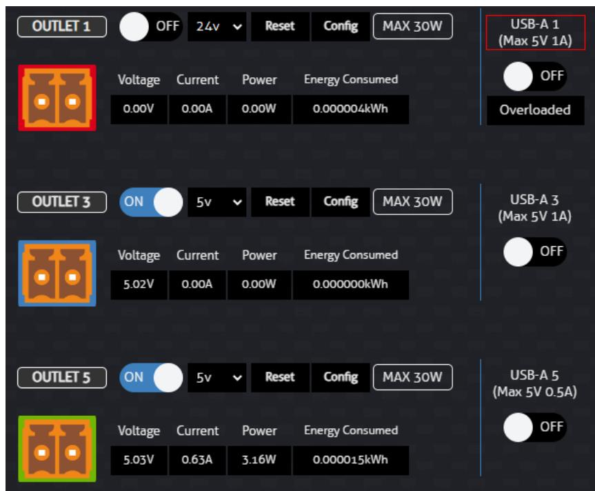
When an outlet of the PWR8VDC enters a warning state, the outlet will be turned off and highlighted in red. This is triggered by abnormal voltage or current on the outlet. When attempting to power on the outlet, a warning dialog will be shown allowing for the warning to be cleared and the outlet to resume normal operation:
