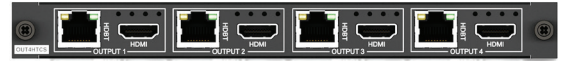
PRO-OUT4HTCS 4-Way Simultaneous HDBaseT™ / HDMI 2.0 Output Board - 4K 60Hz 4:4:4 to 70m (1080p up to 100m)
