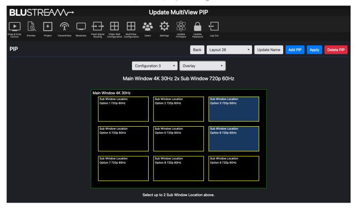
Once the most suitable Configuration has been chosen, select either 'Side by Side' or 'Overlay' from the drop-down box next to the Configuration.
