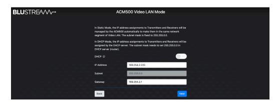
By default, the ACM500 will assign the IP500UHD-TZ IP addresses based on the rules outlined on the next page. Where the IP addresses need to be assigned from a DHCP server, the IP address of the Video LAN port can be adjusted from this page to suit the system.
