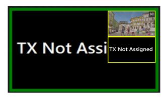
As each source is dropped onto the available window, the thumbnail will appear inside the window. A small button will appear in the corner of the windows. In the green Main Window, MC (Main Clear) will appear, in the yellow Sub Windows, SC (Sub Clear) will appear - clicking these buttons will clear the source assigned to that portion of the screen.
