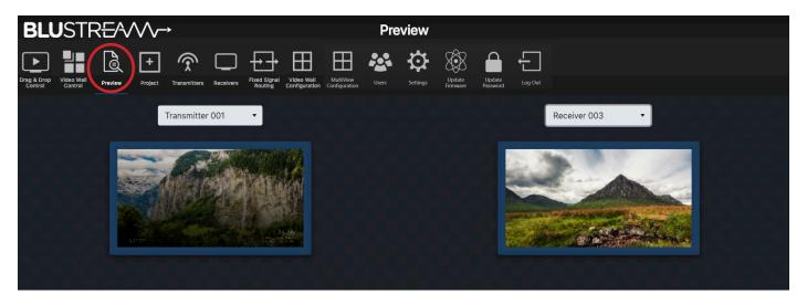
The Preview windows show a live grab of the media which automatically updates every few seconds. To select the Transmitter or Receiver to preview, use the drop down box to select the individual Transmitter or Receiver to preview. Note that if a receiver is in video wall mode, you will receive a message "RX is assigned as part of a video wall". To preview this RX, you would need to first disable the video wall mode.
