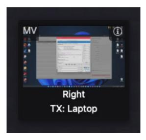
Clicking on the MV symbol for the RX that needs to have a Mulit-View window applied, shows a visual representation of the screen in its current state or layout. The available MultiView presets are able to be selected from the options at the bottom of the window. To select one of the available MultiView options, drag and drop the Preset onto the representation of the screen. The display will immediately change its layout to the selected Preset.
